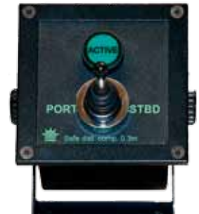
STS Joystick With push button to activate steering position.
